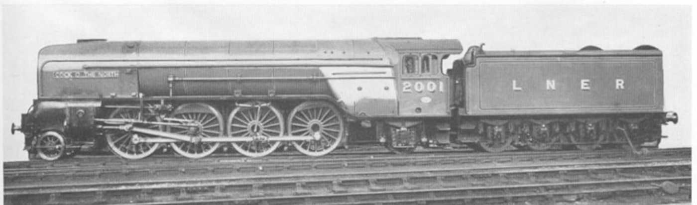
Fig. 10. Sir Nigel Gresley's 2-8-2 Three-Cylinder Passenger Locomotive (1934) with Poppet Valve Gear
