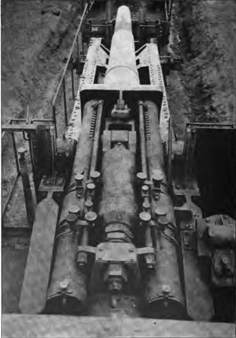
CRADLE, RECOIL CYLINDER, AND SPRING RECUPERATORS OF THE 210-MM.
