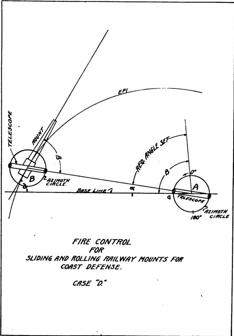
shaft which carried the observation telescope through which the target was being followed. Plate 436 gives a rough sketch of such a scheme.
